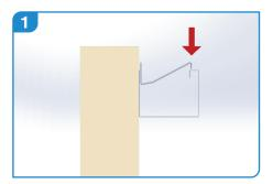
Legion joggle joint guttering is fitted direct to the fascia board at 750 mm centres and has pre-drilled holes for fixing. Start by deciding whether to fit the gutter level or with a fall to 1:600.
