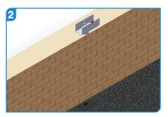
Ideally using a string line or laser level, set out position from bottom edge of gutter.
