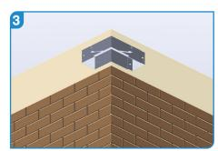
Fix gutter lengths utilising the pre-drilled fixing holes at 750 mm centres in the rear face of the gutter.
