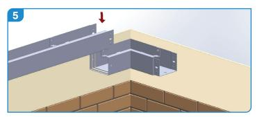
Position the spigot end over the joint, push bolts through the slots of the gutter from the outside, making sure the slotted holes are filled with sealant.
