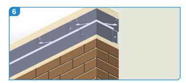
Apply nuts and washers and gently tighten (Do not overtighten as this may force the sealant out of the joint).
