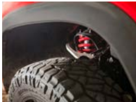
3-in. Suspension Lift Kit 47, 48
