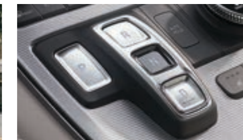
Shift-by-Wire push-button drive controls
