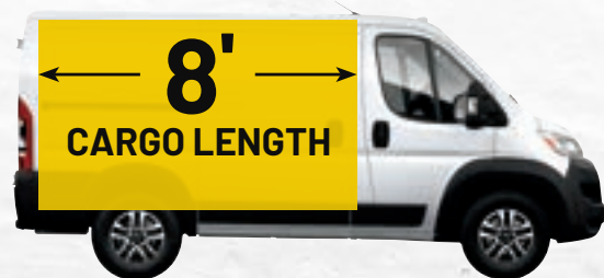
118-INCH WHEELBASE, STANDARD ROOF
