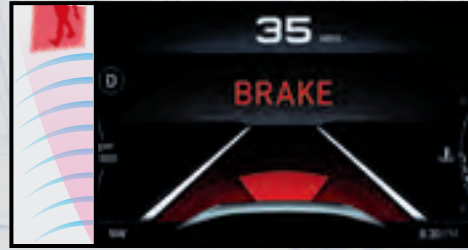
STANDARD FULL-SPEED FORWARD COLLISION WARNING PLUS with PEDESTRIAN/CYCLIST EMERGENCY BRAKING 6
