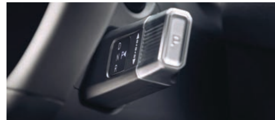
Steering column-mounted Shift-by-Wire gear shifter
