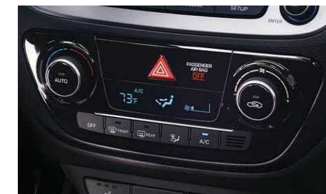
Automatic temperature control
