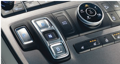
Shift-by-Wire push-button gear selection
