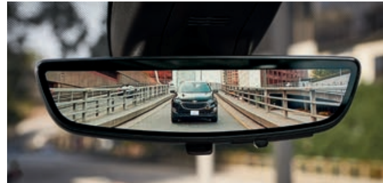
Rear Camera Mirror An available dual-function camera-based rearview mirror provides a wider, less-obstructed field of view than a traditional rearview mirror.
