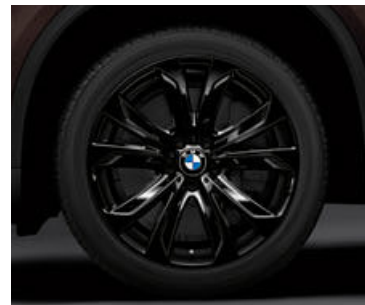
□ 20" light alloy wheels Star-spoke style 491 with mixed tyres, Black high-gloss, front 10 J x 20 with 275/40 R 20 tyres, rear 11 J x 20 with 315/35 R 20 tyres.
