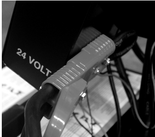
24 Volt Quick Connect (Red) with Voltage Selection Quick Connect Attached
