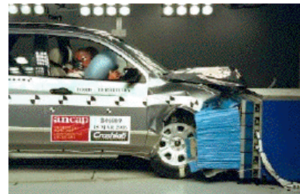
Offset crash test at 64km/h (2006)
