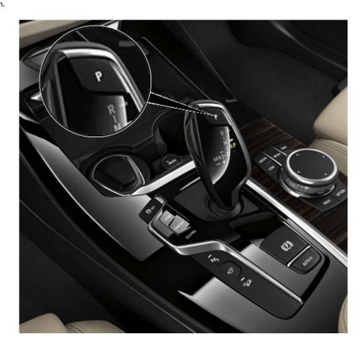
Pull up the switch for the electric parking brake.
