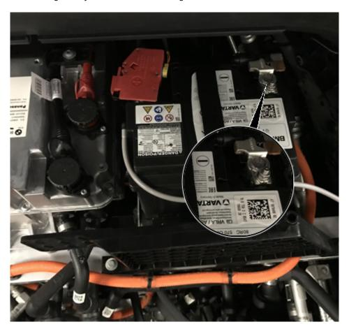
Release the negative battery cable and pull it off upwards.
