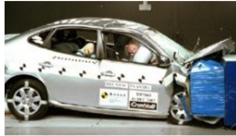
Offset crash test at 64km/hr
