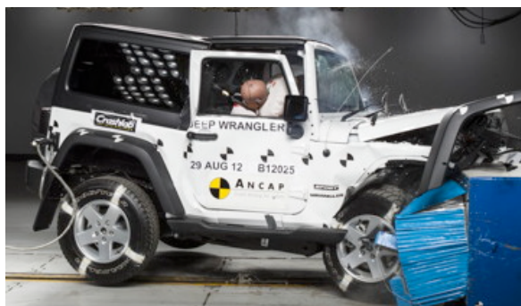
Offset crash test at 64km/h
