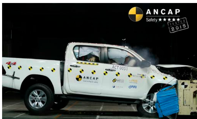
Frontal offset test at 64km/h
