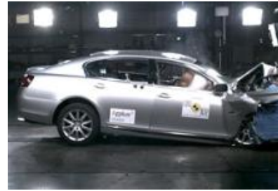
Offset crash test at 64km/hr
