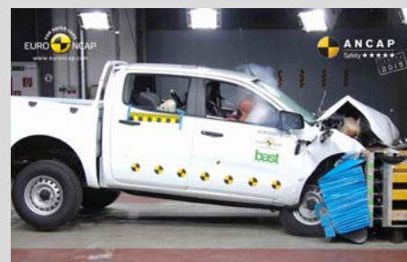
Frontal offset test at 64km/h
