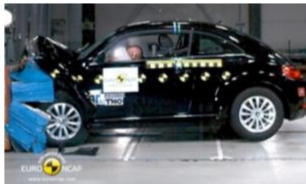
Frontal offset test at 64 km/h
