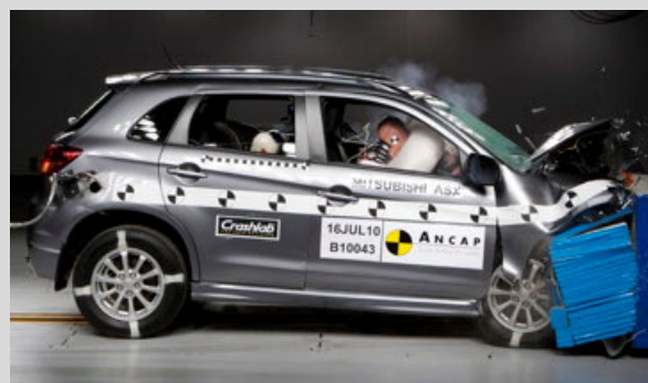
Frontal offset test at 64km/h
