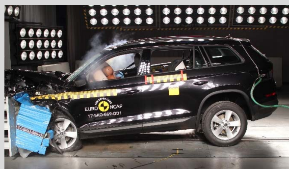
Frontal offset test at 64km/h
