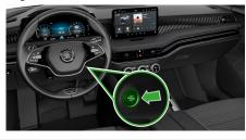
Press the "Engine Start/Stop" button in the centre console without engaging the brake pedal.
