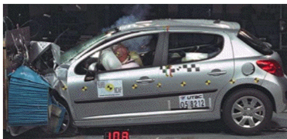
Offset crash test at 64km/h
