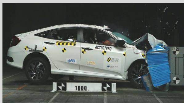
Frontal offset test at 64km/h
