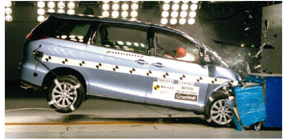
Offset crash test at 64km/h
