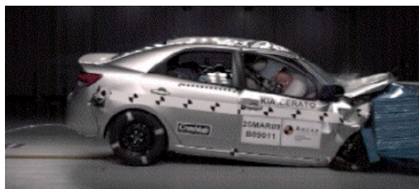
Offset crash test at 64km/h
