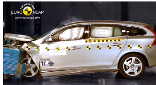
Offset crash test at 64km/h (V60)
