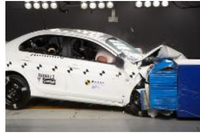
Offset crash test at 64km/hr
