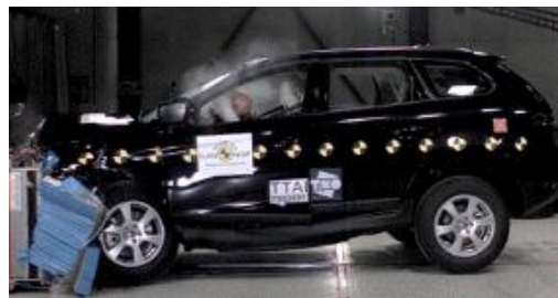
Offset crash test at 64km/hr
