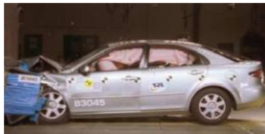
Offset crash test at 64km/hr
