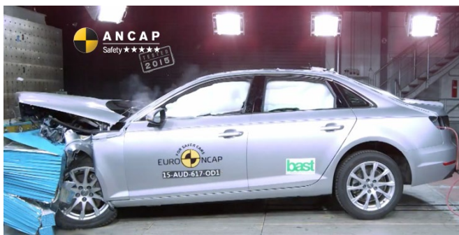
Frontal offset test at 64km/h (copyright Euro NCAP)
