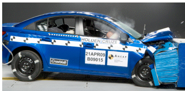
Offset crash test at 64km/h
