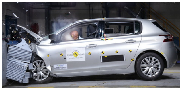
Frontal offset test at 64 km/h (Euro NCAP)
