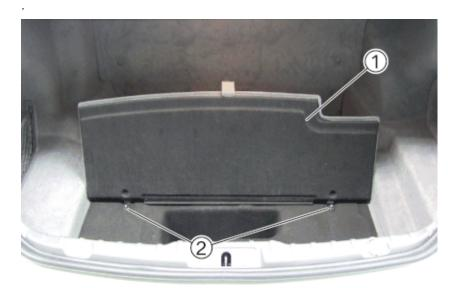
Open the tailgate and fold the luggage compartment floor trim panel (1) up. Loosen plastic nuts (2) and remove luggage compartment floor trim panel (1).
