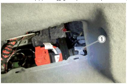
Loosen the nut and pull the battery earth lead (1) off toward the top. Cover the battery earth lead to prevent contact with the battery terminal.
