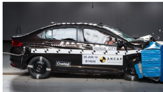
Frontal offset test at 64 km/h
