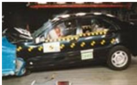
Offset crash test at 64km/hr
