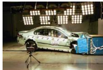
Offset crash test at 64km/hr
