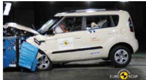
Offset crash test at 64km/hr
