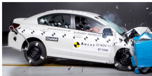
Offset crash test at 64km/h
