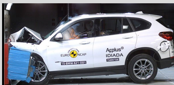
Frontal offset test at 64km/h
