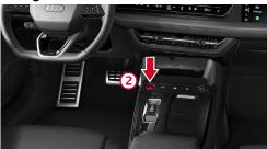
② Switch off ignition (power meter "OFF"), press "Start-Stop" button without operating foot brake.
