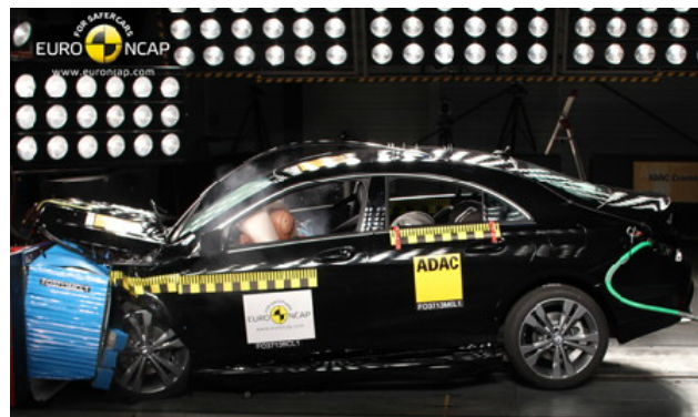
Frontal offset test at 64 km/h (Euro NCAP)
