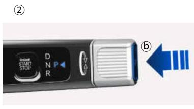
1. Chock the wheels and pull the EPB switch to set the parking brake.
