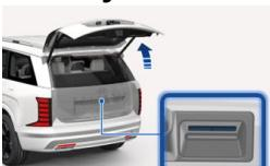
1. Press the power tailgate open/close button for 1 second. The tailgate opens or closes with a warning sound.
