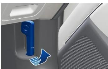
1. Pull the hood release lever to open the hood.
