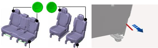
If the walk-in switch does not work, pull the strap located on the lower right side of the seat.
