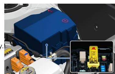
Pull "Service Interlock" upwards.
