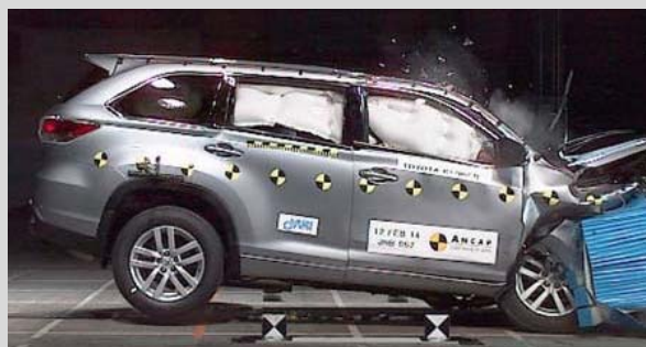
Frontal offset test at 64km/h
