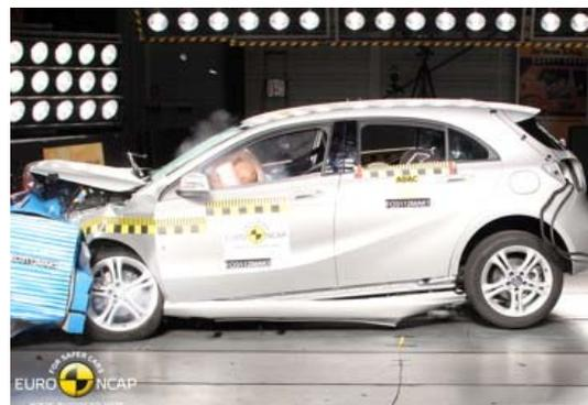
Frontal offset test at 64 km/h (Euro NCAP)
