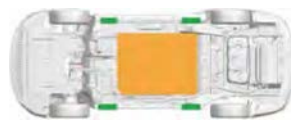
— Stabilisation-lifting points — High voltage battery
