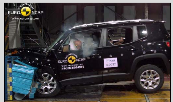
Frontal offset test at 64km/h
