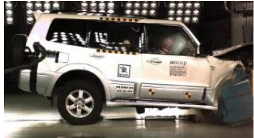
Offset crash test at 64km/hr
