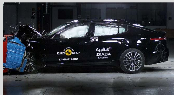
Frontal offset test at 64km/h
