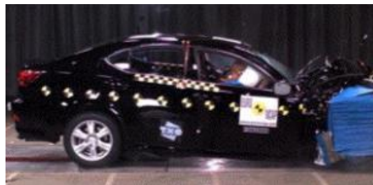
Offset crash test at 64km/hr
